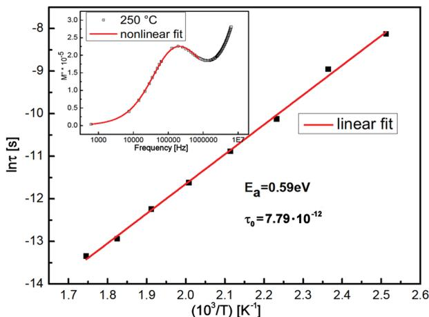
Figure 7. Variation of relaxation time period with temperature obtained from fitting the imaginary part of modulus. Inset figure shows non-linear fit of imaginary part of modulus at 250 °C
