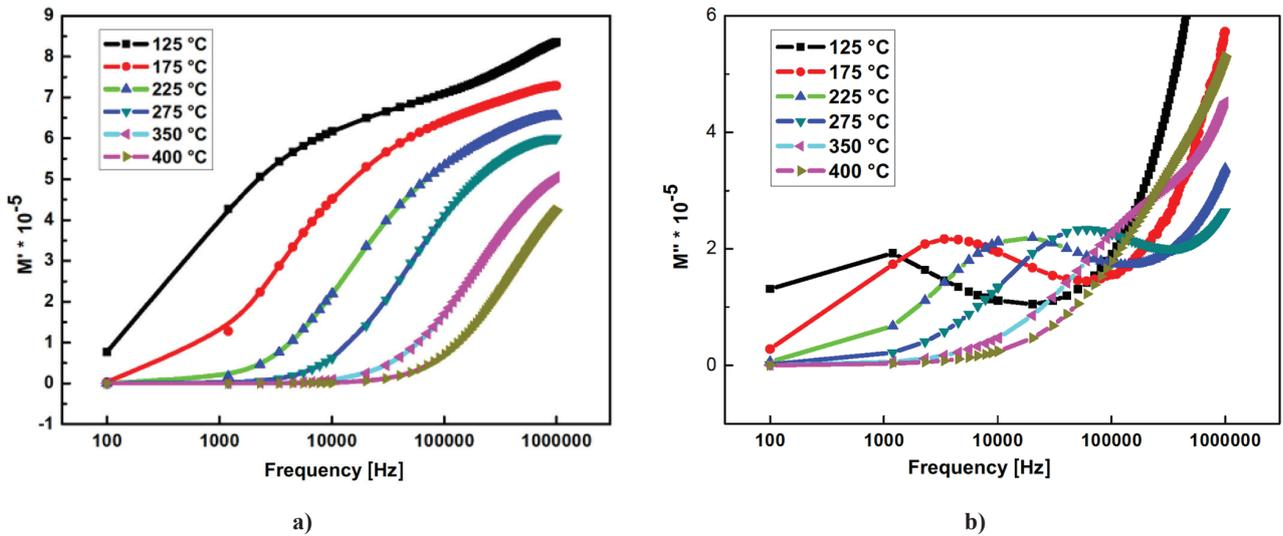
Figure 6. Variation of real (a) and imaginary part (b) of electric modulus with frequency at different indicated measurement temperatures
