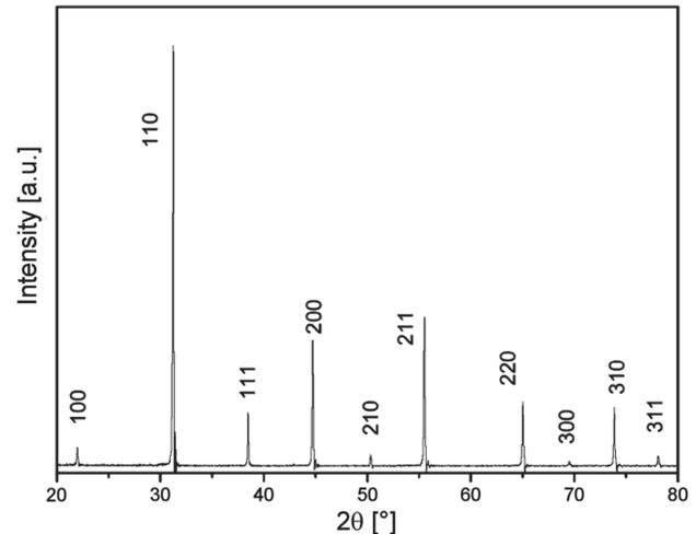
Figure 1. XRD pattern of BFN powder calcined at 1250 °C
