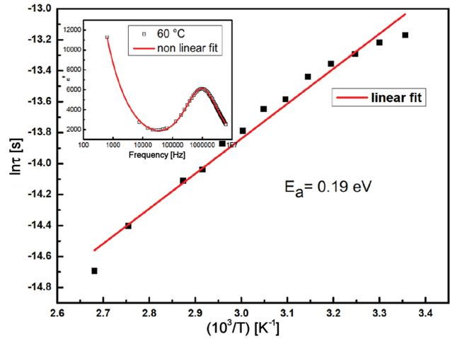
Figure 5. Variation of relaxation time period with temperature. Inset figure shows nonlinear fit of the frequency dependent dielectric loss ( $\epsilon''$ ) at 60 °C
