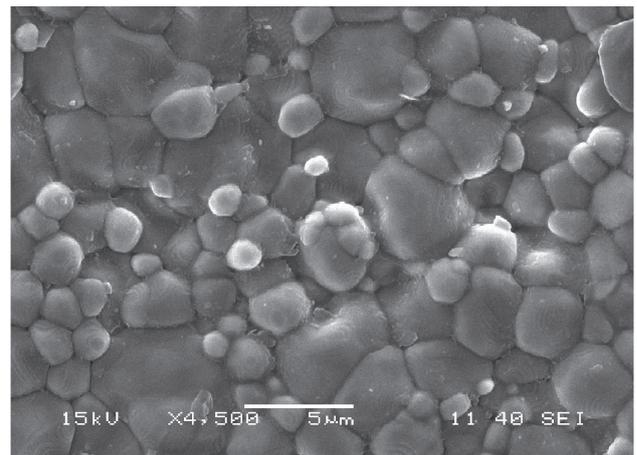
Figure 2. SEM of BFN ceramic sintered at 1350 °C
