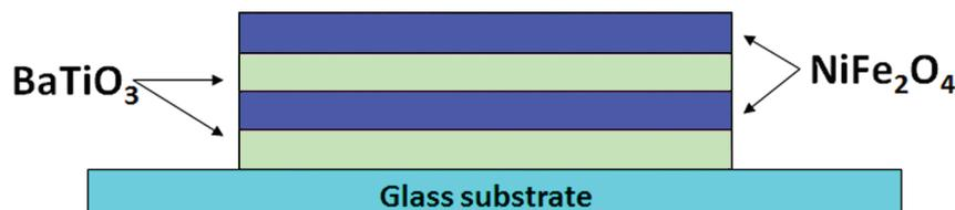
Figure 1. Schematic representation of multilayered BaTiO<sub>3</sub>/NiFe<sub>2</sub>O<sub>4</sub> thin films
