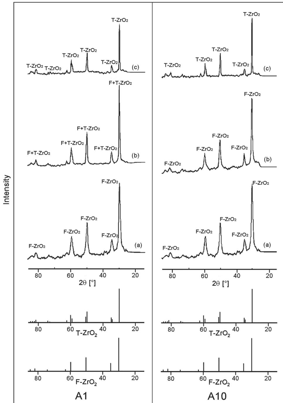
Figure 1. XRD patterns of A1 and A10 nanocrystalline powders after hydrothermal treatment at 210 °C (a) and heat treatment at temperature 900 °C (b) and 1200 °C (c)
