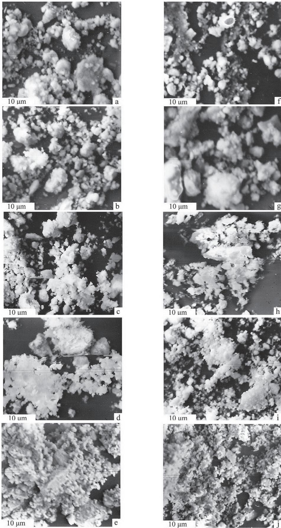
Figure 2. SEM images showing the nanocrystalline powders A1 (a-e) and A10 (f-j): after hydrothermal treatment (a,f) and heat treatment at 500 °C (b,g), 700 °C(c,h), 900 °C(d, i) and 1200 °C (e,j)
