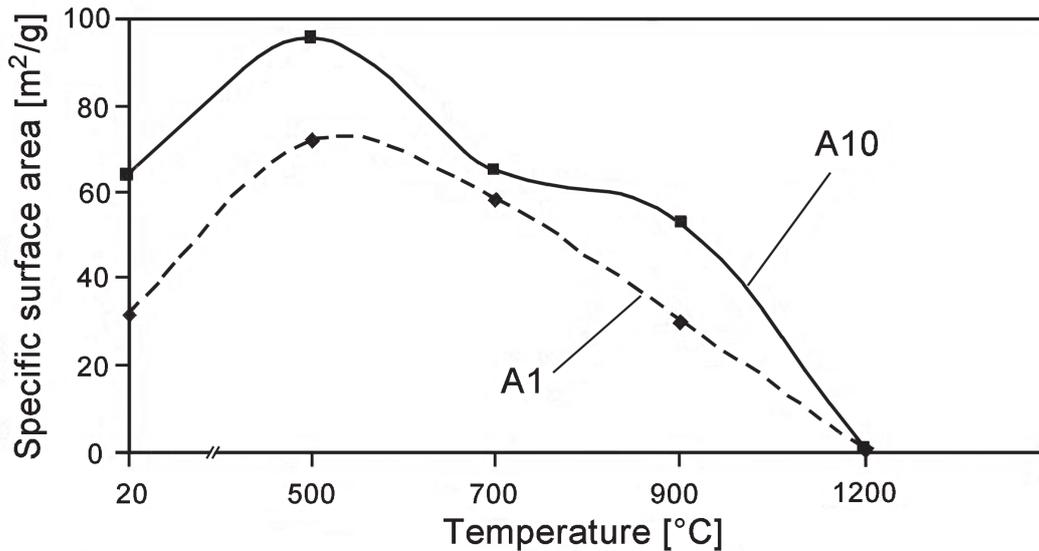
Figure 3. Effect of heat treatment on the specific surface area of the nanocrystalline  $ZrO_2$ - $Y_2O_3$ - $CeO_2$ - $CoO$ - $Al_2O_3$  powders
