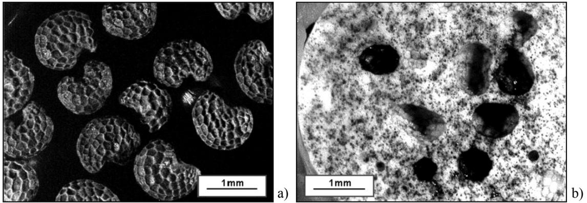
Figure 5. Optical micrograph of poppy seed (left) and microstructure of porous alumina ceramics prepared with poppy seed (polished section, right)
