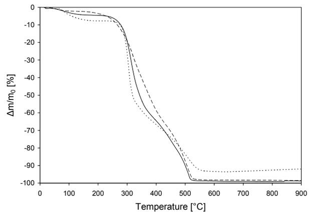
**Figure 10. Thermogravimetric (TG) curves of lycopodium (dashed line), coffee (full line) and semolina (dotted line) measured with a heating rate of 10°C/min in air atmosphere**
