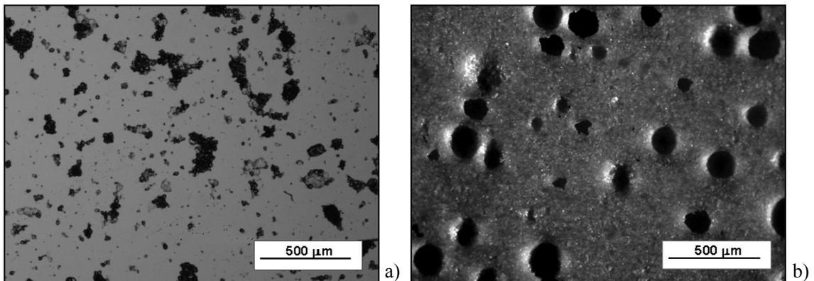
Figure 7. Optical micrograph of fine flour (left) and microstructure of porous alumina ceramics prepared with fine flour (polished section, right)
