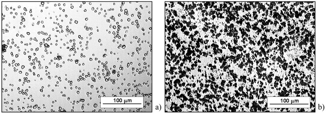
Figure 1. Optical micrograph of rice starch (left) and microstructure of porous alumina ceramics prepared via SCC with 10 vol% rice starch (polished section, right)
