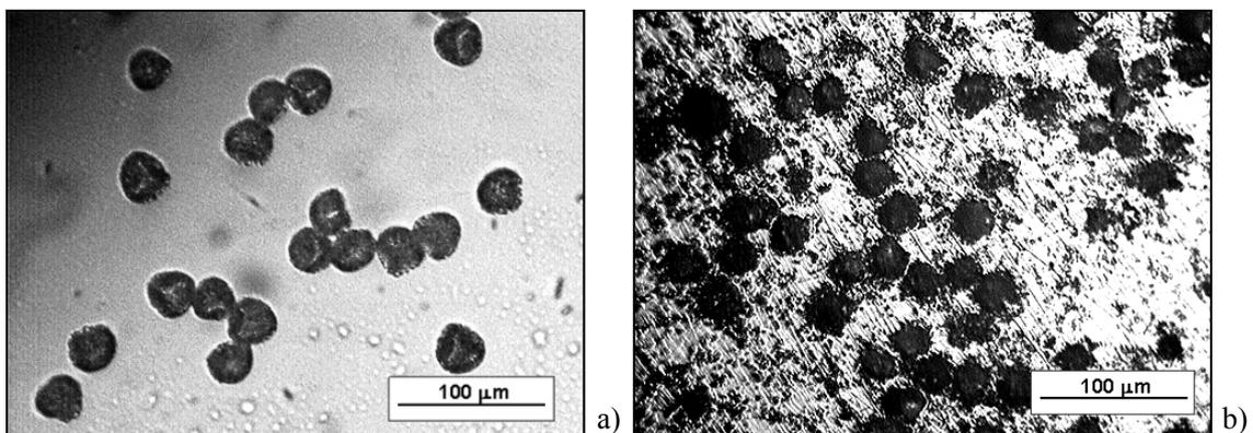
Figure 4. Optical micrograph of lycopodium (left) and microstructure of porous alumina ceramics prepared with 10 vol% lycopodium (polished section, right)
