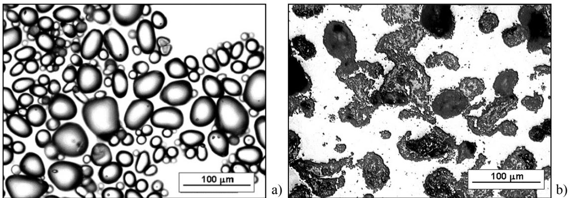
Figure 3. Optical micrograph of potato starch (left) and microstructure of porous alumina ceramics prepared via SCC with 10 vol% potato starch (polished section, right)
