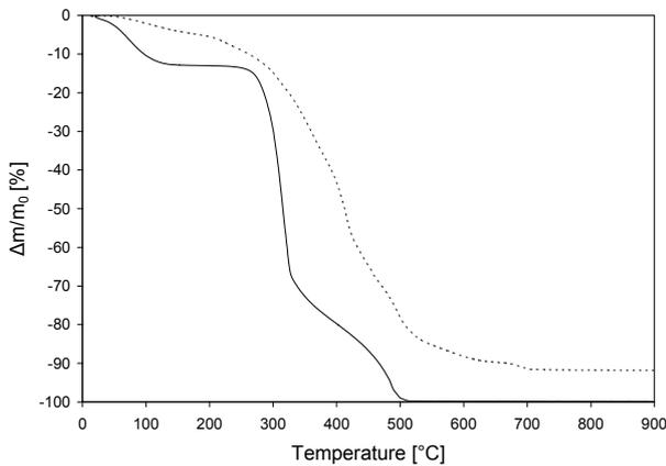
**Figure 9. Thermogravimetric (TG) curves of starch (full line) and poppy seed (dotted line) measured with a heating rate of 10°C/min in air atmosphere**
