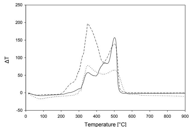
**Figure 12. Differential thermal analysis (DTA) curves of lycopodium (dashed line), coffee (full line) and semolina (dotted line) measured with a heating rate of 10 °C/min in air atmosphere**
