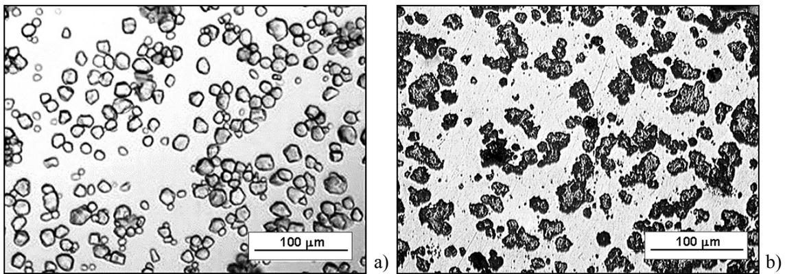
Figure 2. Optical micrograph of corn starch (left) and microstructure of porous alumina ceramics prepared via SCC with 10 vol% corn starch (polished section, right)
