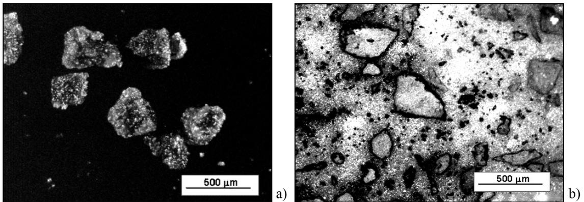
Figure 6. Optical micrograph of coffee (left) and microstructure of porous alumina ceramics prepared with coffee (polished section, right)
