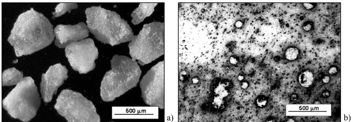
Figure 8. Optical micrograph of semolina (left) and microstructure of porous alumina ceramics prepared with semolina (polished section, right)
