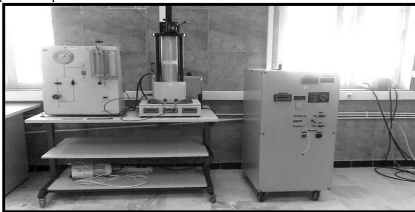
Figure 5. Flash separation equipment and DBROBINSON brand gasometer
