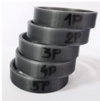
Figure 3. Pipe Ring Notched Tensile specimens.
