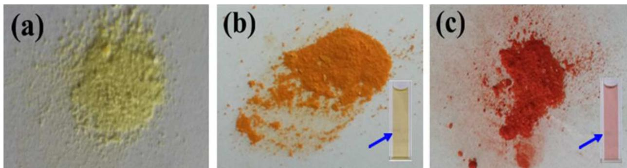
**Figure 10.** Digital photograph of : (a) powdered  $\text{CeO}_2$  before used, (b) powdered  $\text{CeO}_2$  after used for AO-10 adsorption (inset 15 mg/l of AO-10 dye solution), and (c) powdered  $\text{CeO}_2$  after used for CR adsorption (inset 15 mg/l of CR dye solution) for 120 min of reaction time
