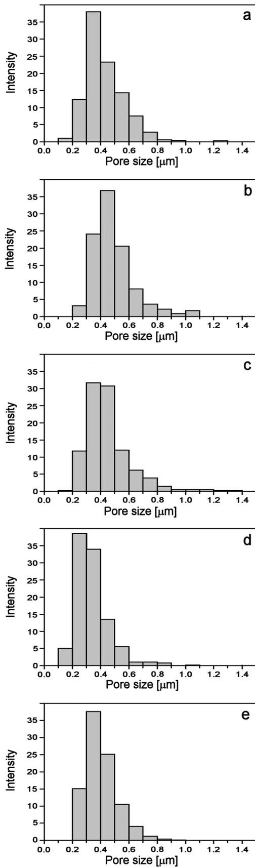
Figure 4. Pore size distribution for BHA samples sintered at 1000 °C for: a) 5, b) 10, c) 15, d) 20 and e) 30 min
