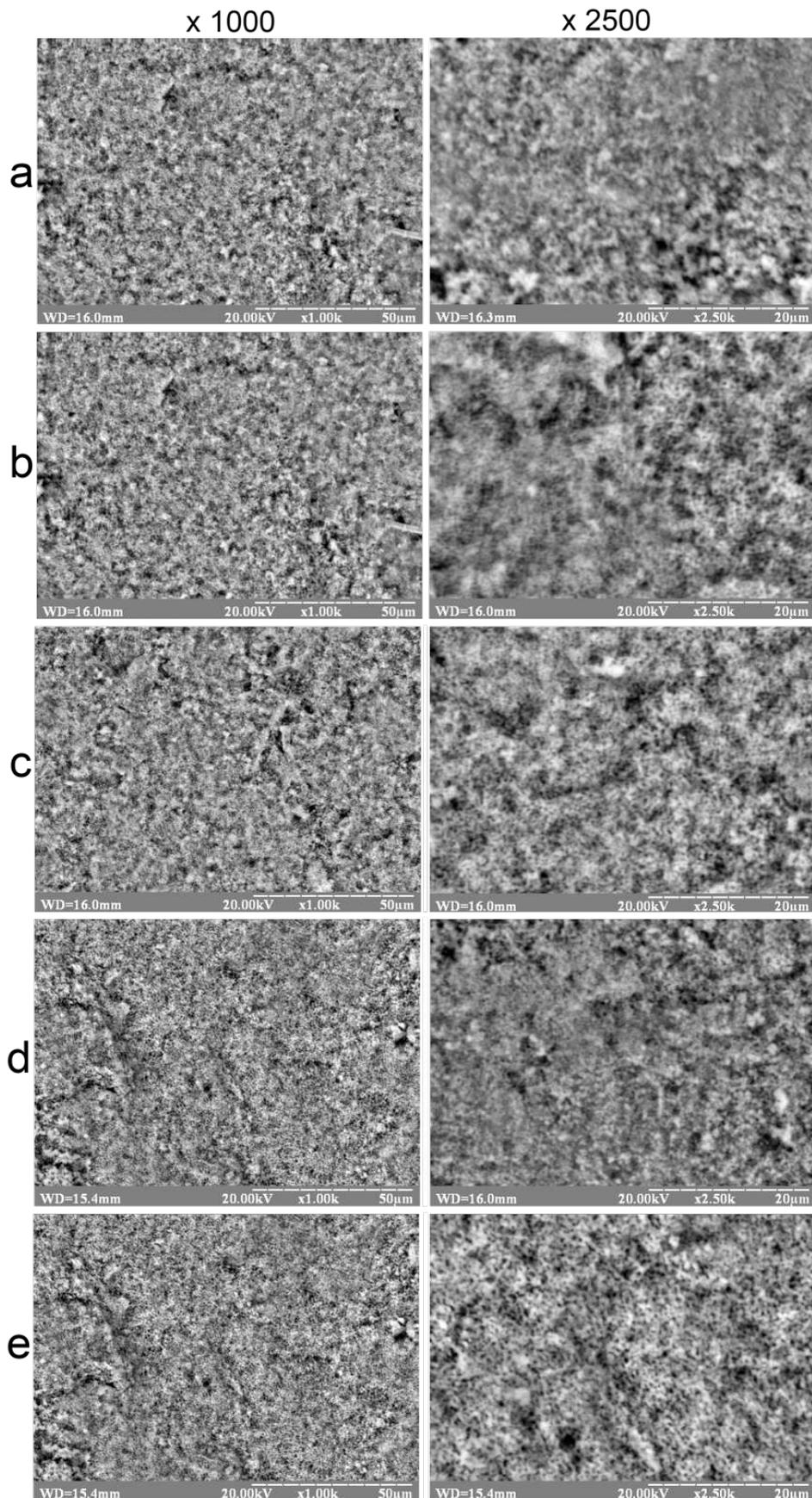
Figure 3. SEM of BHA samples after microwave sintering at 1000 °C for different sintering time: a) 5, b) 10, c) 15, d) 20 and e) 30 min
