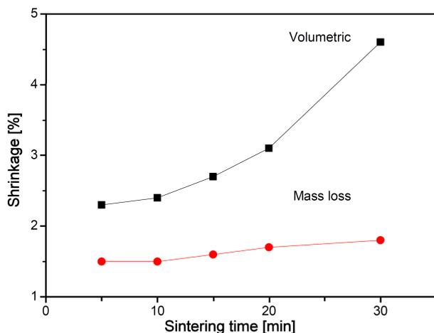
Figure 2. The effect of sintering time on the volumetric shrinkage and weight loss of BHA samples under microwave sintering at 1000 °C
