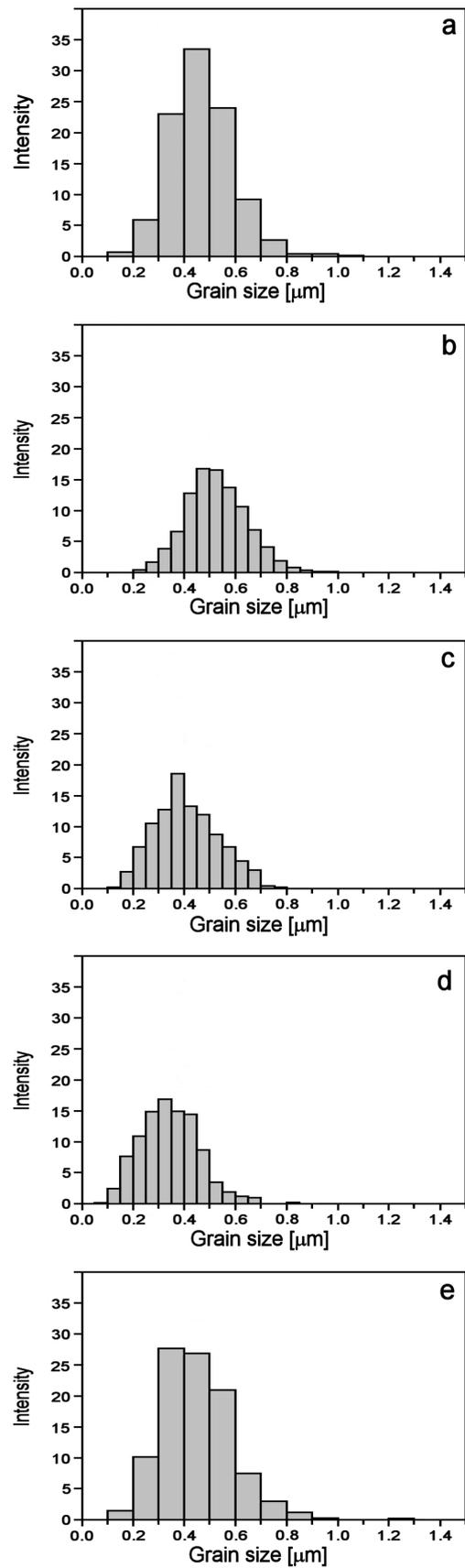
Figure 5. Grain size distribution for BHA samples sintered at 1000 °C for: a) 5, b) 10, c) 15, d) 20 and e) 30 min
