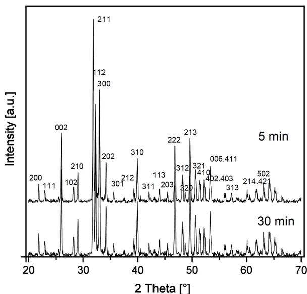
Figure 1. Typical XRD pattern of BHA after microwave sintering at 1000 °C for 5 and 30 min
