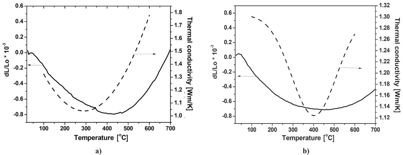
Figure 2. Thermal expansion and thermal conductivity versus temperature for samples: a) AT and b) TAT-5
