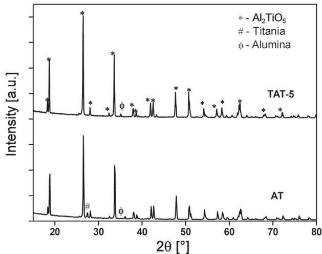
Figure 1. XRD patterns of AT and TAT-5 samples sintered at 1550 °C
