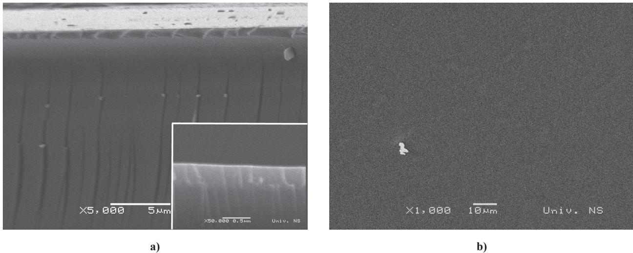
Figure 6. SEM micrographs of multilayered  $\text{BaTiO}_3/\text{NiFe}_2\text{O}_4$  film S2-FT (prepared by spin-coating and drying/annealing of every deposited layer): a) cross section and b) surface morphology
