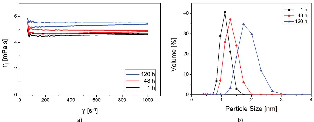
Figure 3. Viscosity (a) and particle size distribution (b) of titanate AT sol
