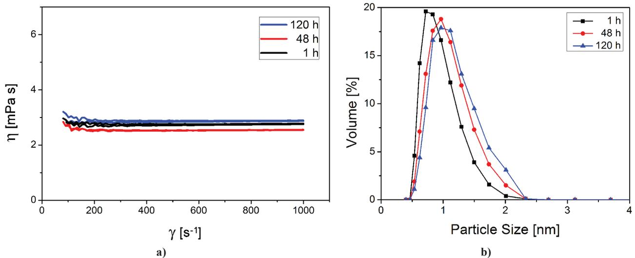
Figure 2. Viscosity (a) and particle size distribution (b) of ferrite MF sol
