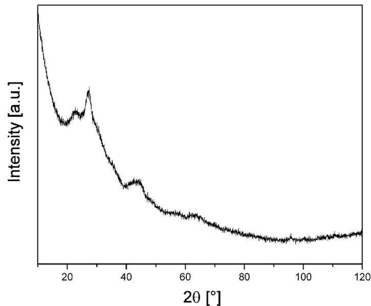
Figure 7. XRD pattern of multilayered  $\text{BaTiO}_3/\text{NiFe}_2\text{O}_4$  film S2-FT (prepared by spin-coating and drying/annealing of every deposited layer)
