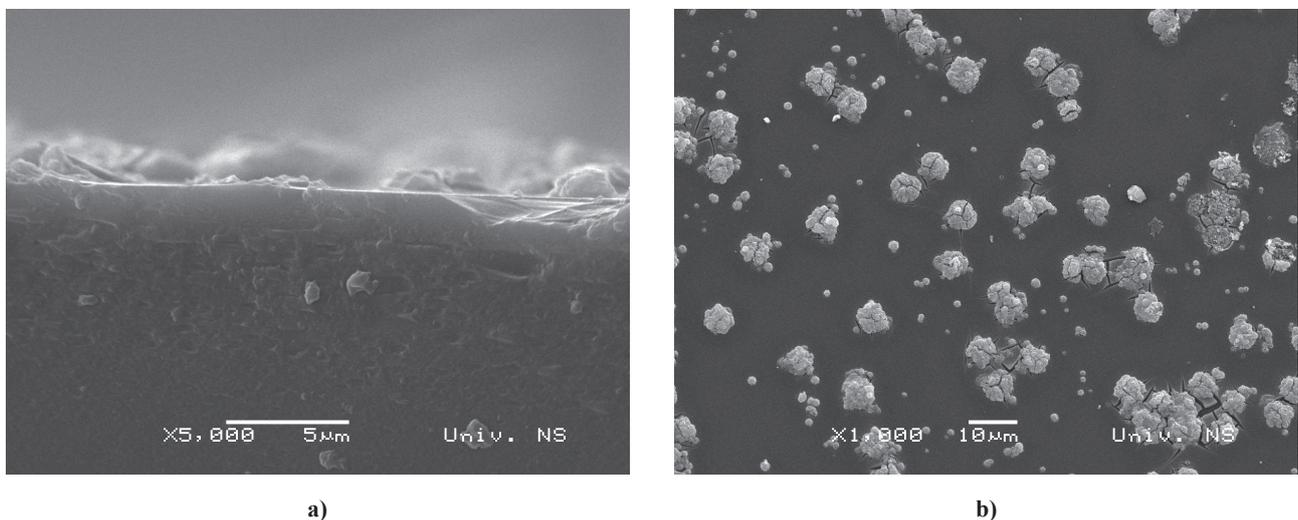
Figure 5. SEM micrographs of multilayered  $\text{BaTiO}_3/\text{NiFe}_2\text{O}_4$  film S1-FT (prepared by spin-coating and drying of every deposited layer): a) cross section and b) surface morphology
