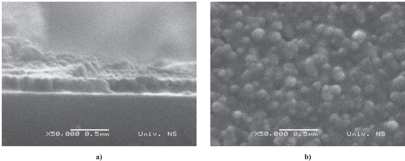
Figure 4. Single ferrite layer deposited by the growth method and calcined at 500 °C for 1 h: a) cross section b) and surface morphology
