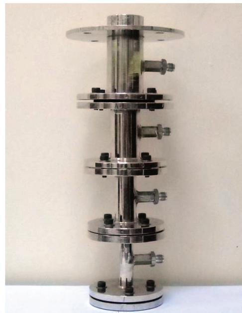
Figure 2. Schematic (a) and photograph (b) of the diffusion burner used in the flame synthesis
