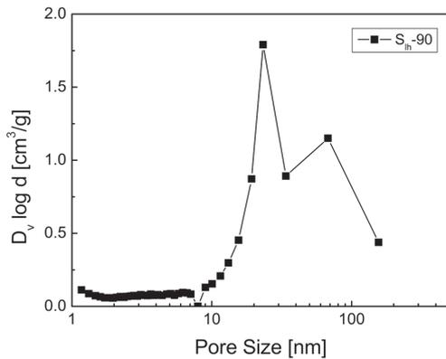
Figure 7. Pore size distribution of silica powder  $S_{ih-90}$
