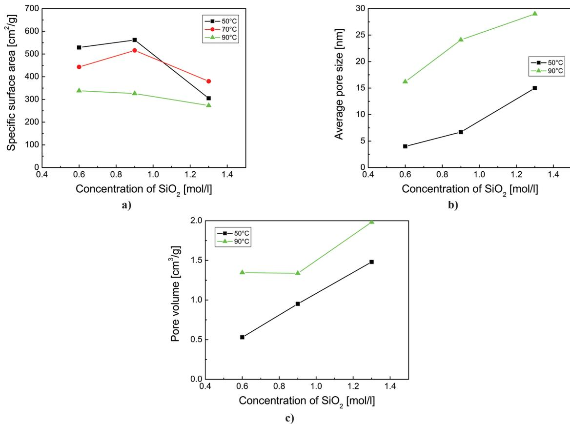
Figure 6. Specific surface area (a), average pore size (b) and pore volume (c) of silica powders synthesized from sodium silicate solutions with different silica concentration and low silica modulus
