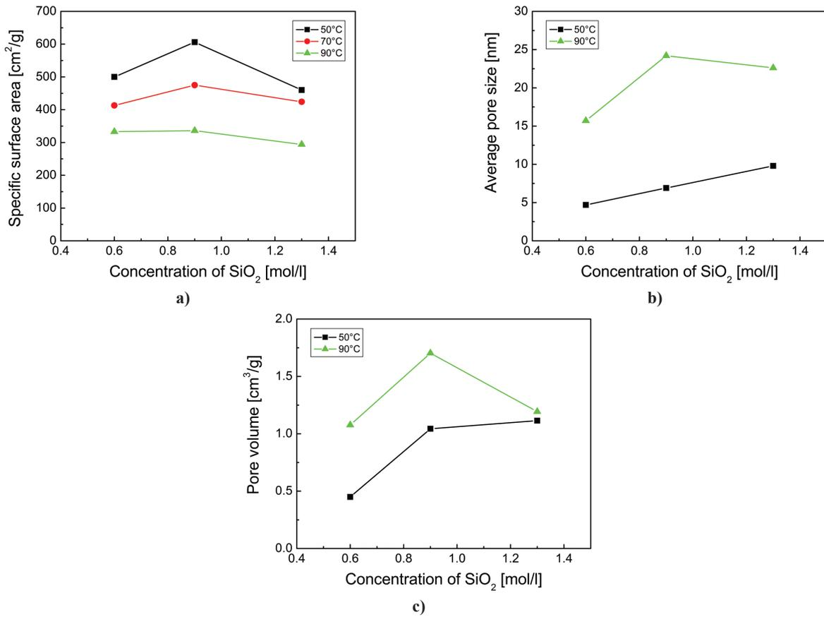
Figure 5. Specific surface area (a), average pore size (b) and pore volume (c) of silica powders synthesized from sodium silicate solutions with different silica concentration and medium silica modulus
