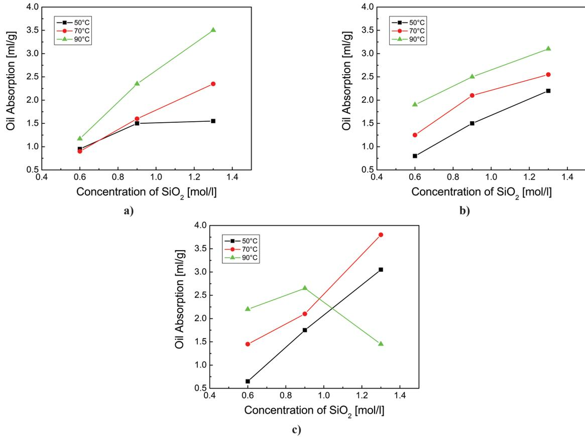
Figure 3. Oil absorption in silica powders synthesized from sodium silicate solutions with different silica concentration: a) high, b) medium and c) low silica modulus
