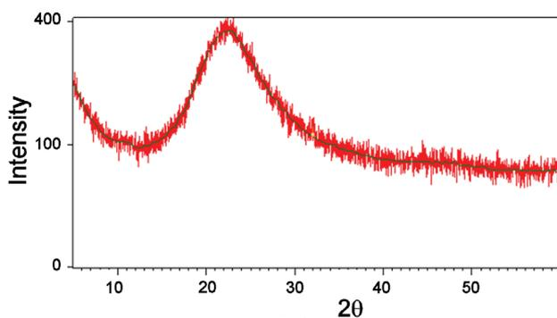
Figure 1. XRD of as-synthesized silica powder
