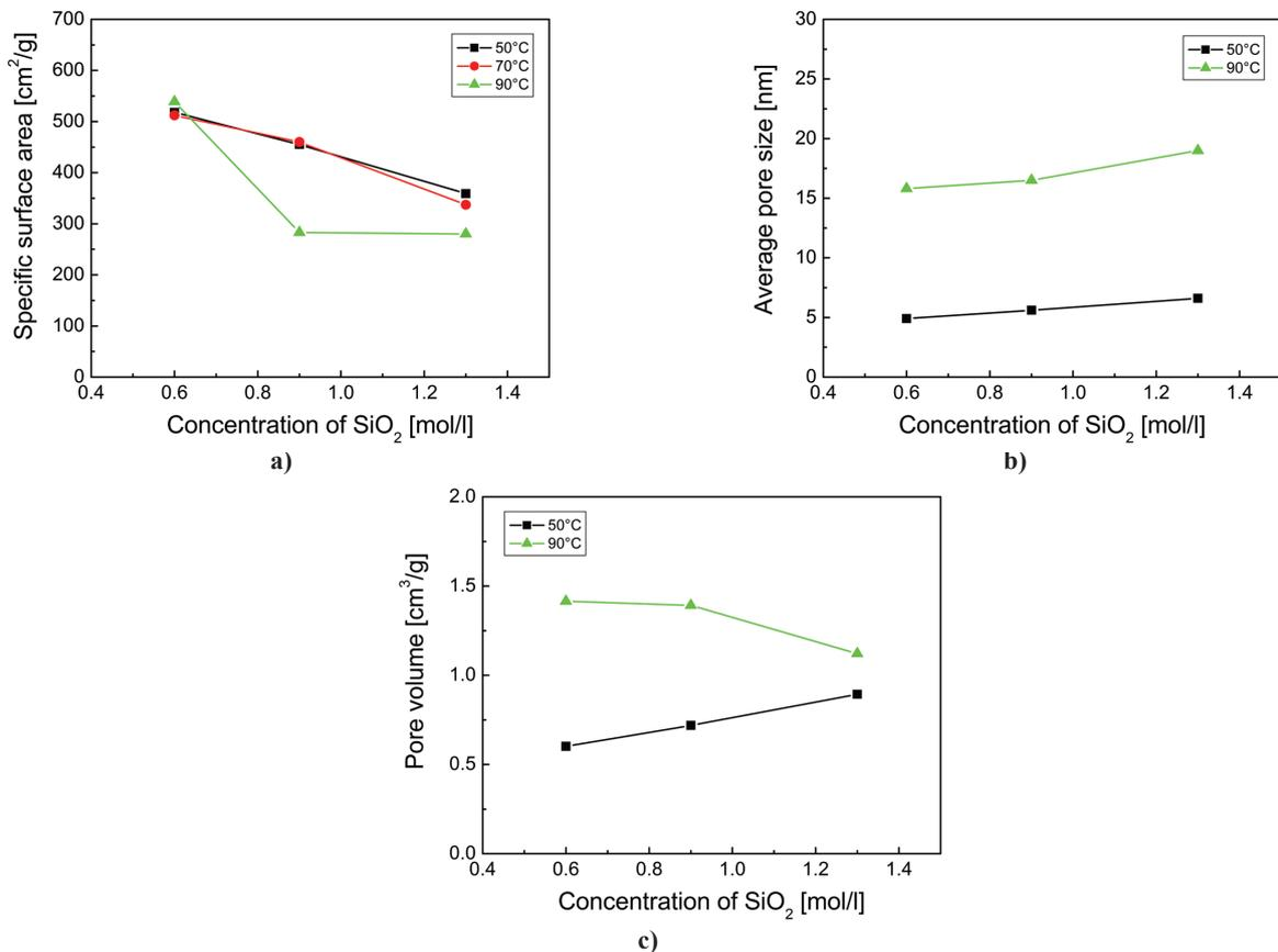
Figure 4. Specific surface area (a), average pore size (b) and pore volume (c) of silica powders synthesized from sodium silicate solutions with different silica concentration and high silica modulus
