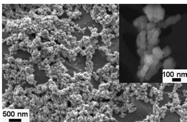
Figure 9. Microstructure (by SEM) of the sample prepared in the presence HPMC at high concentration illustrating the various BaTiO<sub>3</sub> particles morphologies
