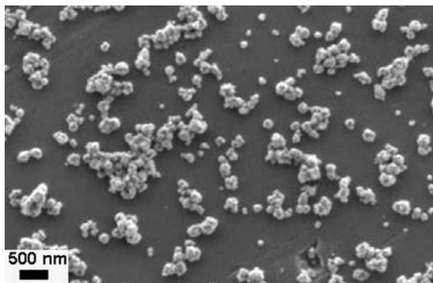
**Figure 7. Microstructure (by SEM) of the sample prepared in the presence PVP at high concentration illustrating disperse and homogeneous BaTiO<sub>3</sub> particles**
