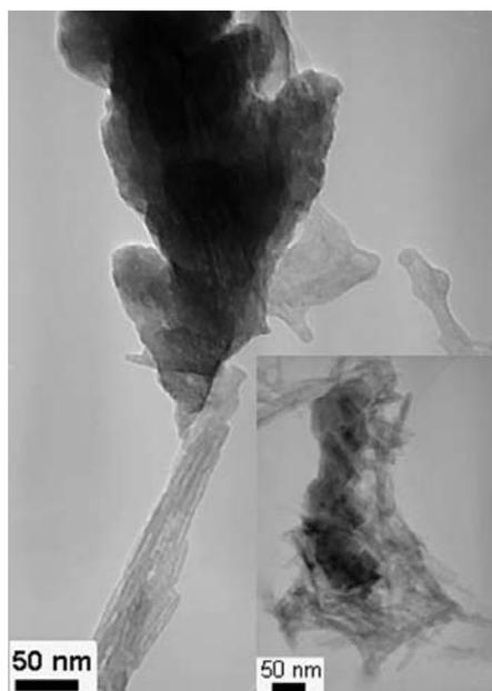
**Figure 2.** TEM micrograph of a sample prepared at the early stages of the reaction at 110°C illustrating the nucleation of BaTiO<sub>3</sub> on the TiNTs surface. In the inset a similar sample prepared at 200°C
