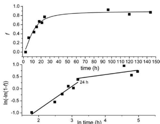
**Figure 1. a) The BaTiO<sub>3</sub> crystalline fraction ( $f$ ) as a function of the synthesis time,  $t$  for the samples prepared by hydrothermal treatment starting from TiNTs at 110°C and b) the corresponding Johnson-Mehl Avrami plot**
