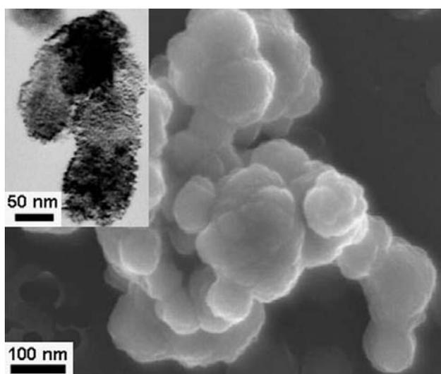
Figure 6. Microstructure (by SEM) of the sample prepared in the presence PAA at high concentration illustrating the oriented attachment and porous feature of BaTiO<sub>3</sub> particles
