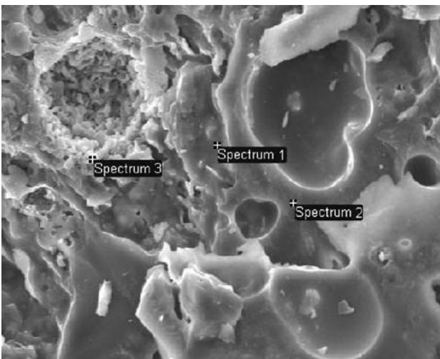
Figure 10. SEM micrograph and EDS spectrums (1-3) of the modified body, T_{firing} 1010^{\circ}\text{C}
