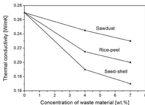
Figure 5. Thermal conductivity of the brick clay samples with different pore-forming additives
