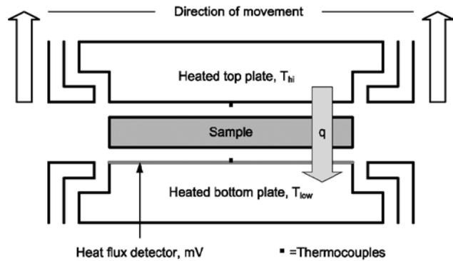
Figure 2. Schematic view of the heat conductivity measuring system
