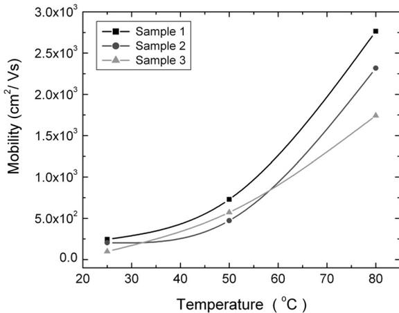
Figure 4. The mobility ( $\mu$ ) as a function of temperature for three analyzed samples
