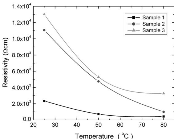
Figure 5. Relationship between the electrical resistivity ( $\rho$ ) and temperature for three samples
