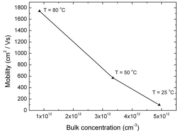
Figure 6. Mobility as a function of the bulk concentration varied with temperature for sample 3
