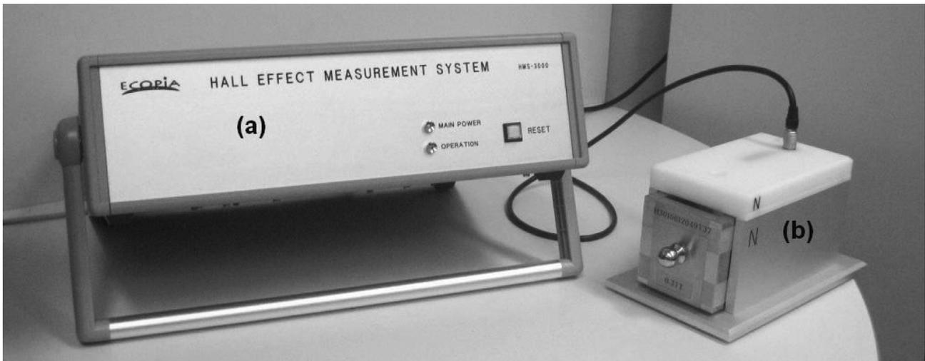
Figure 2. Hall effect measurement system HMS-3000
