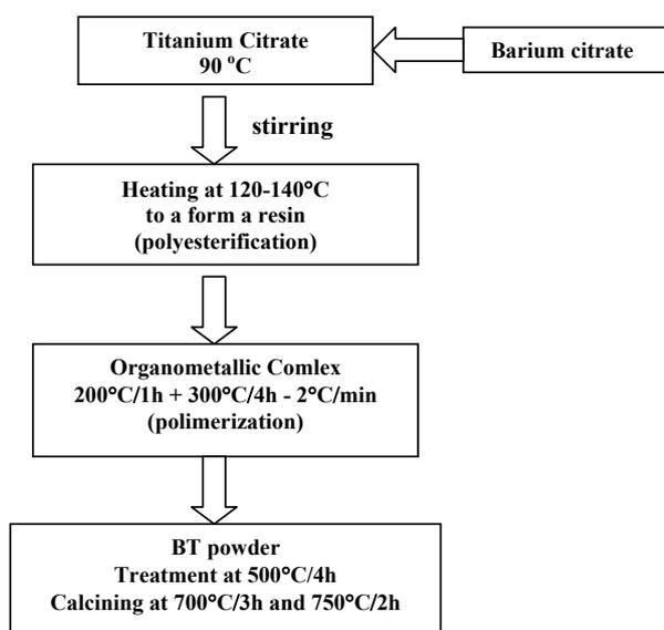
Figure 1. The flow chart for the Pechini process
